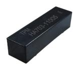
The HA703 series provides a small form factor size of 65.5x15.0mm. It is designed with standard signal pins and coil pins layout. The HA703 series also has coil voltage options of 5.0/12.0/24.0V and dielectric strength options of 10.0/15.0KV and can be adopted to meet our customer's specific design requirements.
